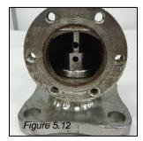
Lift seal disc and install seal disc bolt, apply thread locker to seal disc bolt threads before installation.
