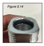
9. Thread packing screw into body, square end up then tighten. Leave 2 to 3 threads below square ends (Figure 5.15 & 5.16)
