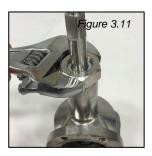
7. Loosen and remove the packing screw using an adjustable wrench. Remove O-ring from packing screw using a hook and pick. (Figure 3.12, 3.13 & 3.14)
